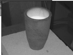
Preparation of a crucible melt in a laboratory furnace at 1350 °C
