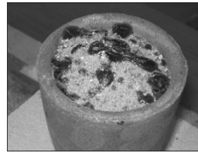
After charging soak time 2 minutes 1250 °C - surface glazed
